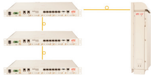
tHost units can be cascaded and their signals are digitally processed and combined
